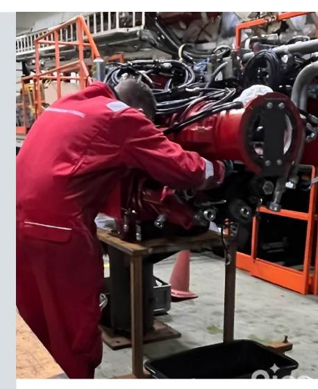
Our expert mechanics quickly diagnosed the problem - worn main shaft bearings - and discovered other top drive parts that needed replacing. With the clock ticking, the team worked at full speed, securing the necessary parts and completing a complex rebuild in just 1.5 weeks!
